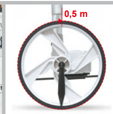
Metering wheel with 0,5-metre circumference
